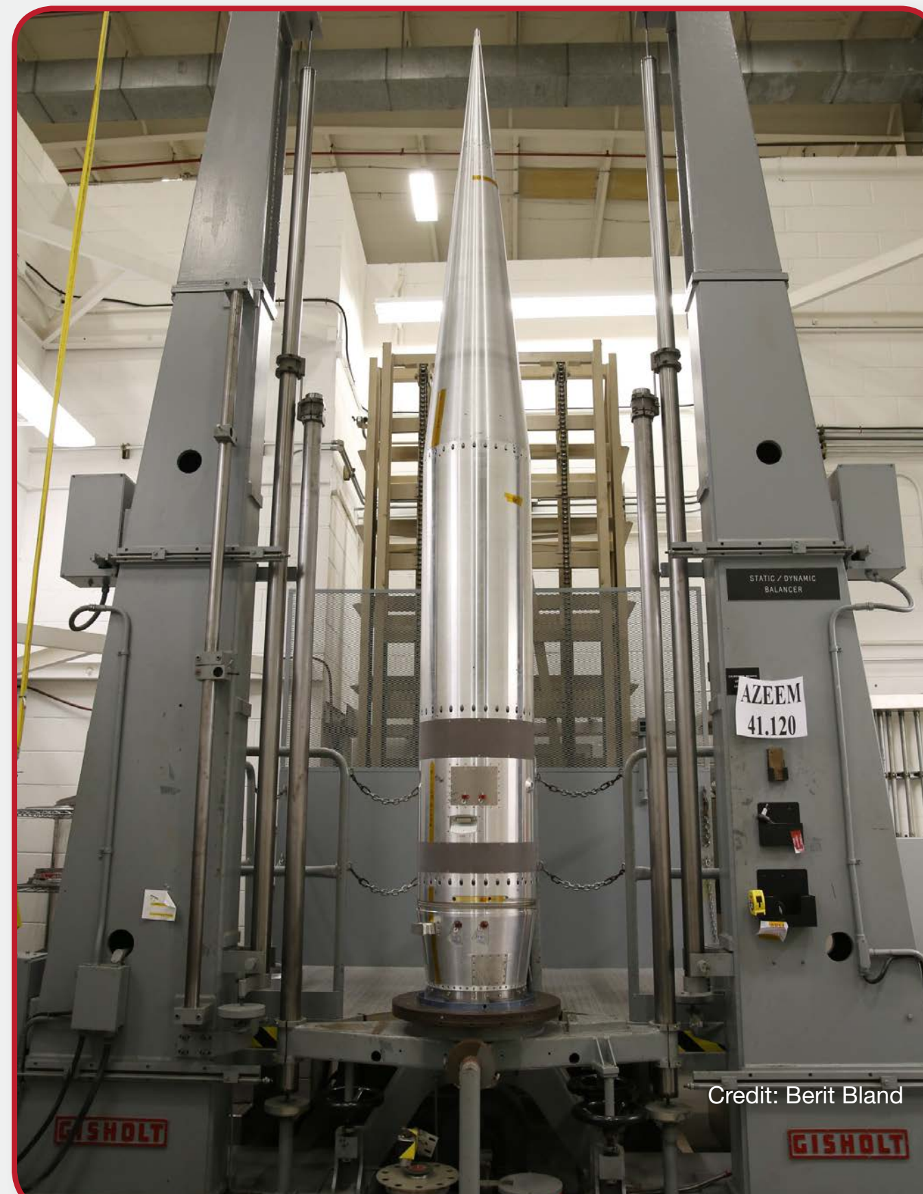
One of the three Super Soaker payloads undergoes spin/balance testing in the Sounding Rocket Payload Processing Facility at NASA's Wallops Flight Facility.
