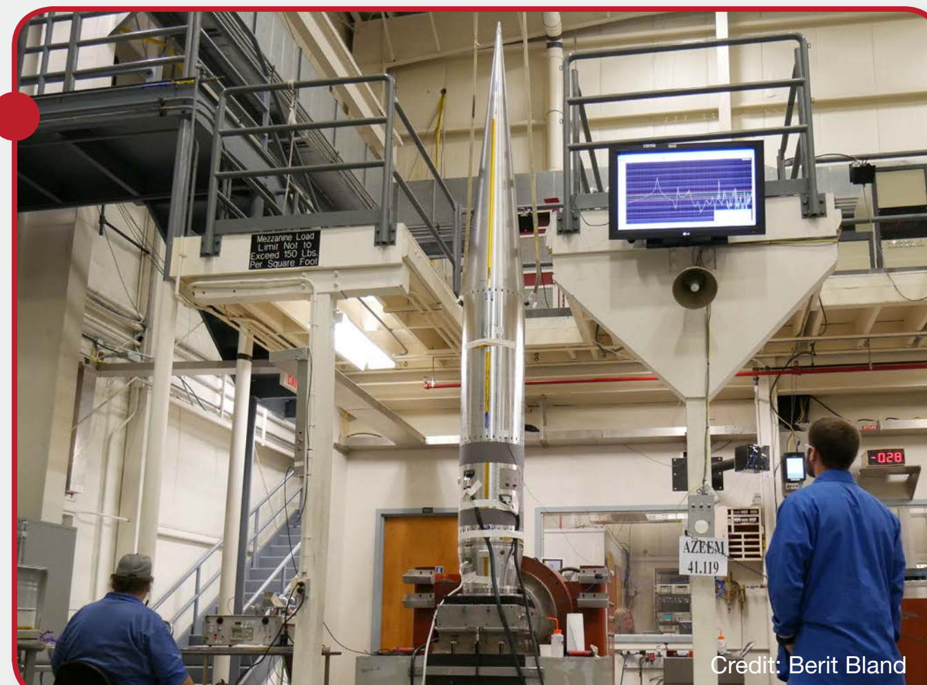
A Super Soaker payload is tested for its ability to operate while experiencing vibrations during flight.
