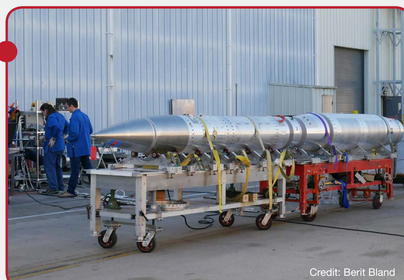
Personnel at the Wallops Flight Facility test the DXL payload's ability to connect with the Global Positioning Satellite (GPS) network which will be used to determine the location of the payload during flight.
