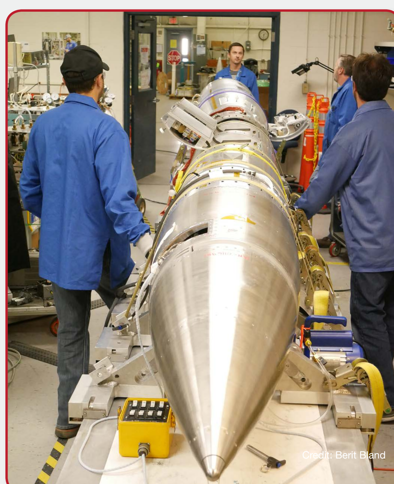
The DXL payload is assembled at NASA's Wallops Flight Facility in Virginia prior to its shipment to the Poker Flat Research Range in Alaska.
