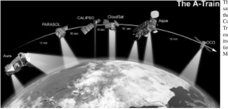
This graphic shows the satellites that make up the Afternoon Constellation—"The A-Train." Listed under each satellite's name is its equator crossing time. (Credit: Alex McClung)
